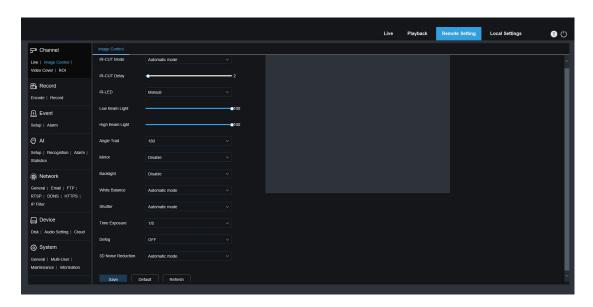
**IR-CUT Mode:** Set the day/night switching mode of the camera, a total of 5 modes.
