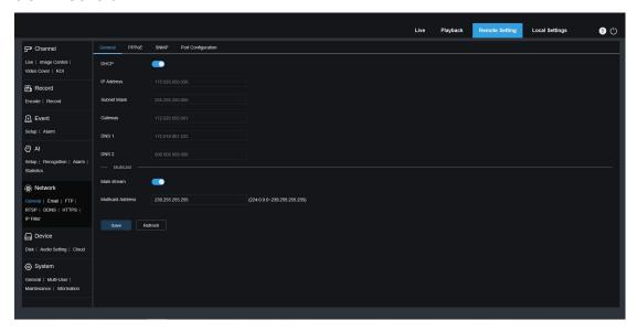
If connecting to a router that allows the use of DHCP, check the DHCP box. The router will automatically assign all network parameters to the camera unless you manually set the following parameters for the network:
