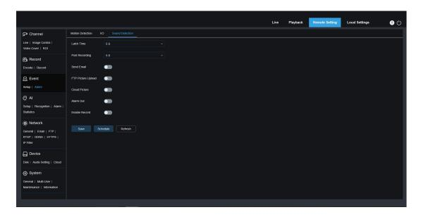
**Latch Time:** Set the external alarm triggering time when motion is detected.
