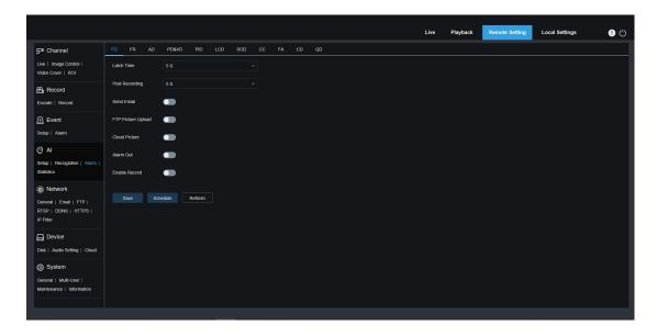
**Alarm Type:** Special option for AD alarm. The camera can alarm by identifying whether the captured object is wearing a mask or not. There are 3 modes.
